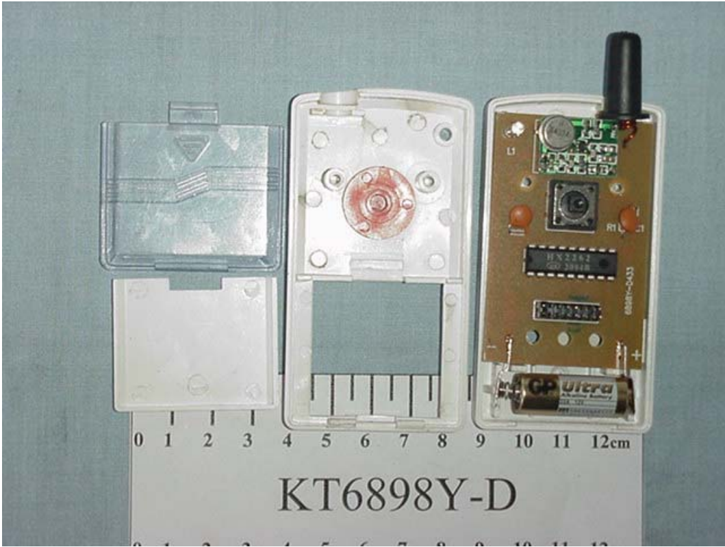
FIGURE 1 WIRELESS DOOR CHIME (M/N: KT6898Y-D) COVER REMOVED
