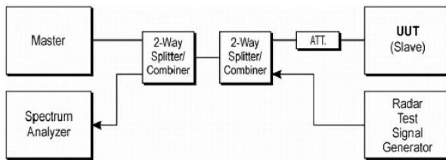
Figure 3-1. Conducted Test Setup for DFS
