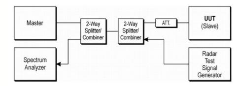
Figure 3-1. Conducted Test Setup for DFS
