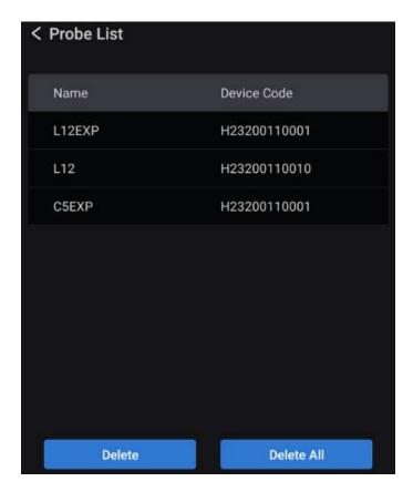
All the probes that have been connected will be shown in this list, you can delete the connected probes one by one, or press **Delete All** button to delete all the connected probes with one click.
