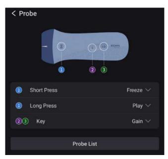
There are three buttons on the body of the Nano Probe, namely buttons ①, ② and ③. User can define the functions of the three buttons for quick operation according to their needs.
