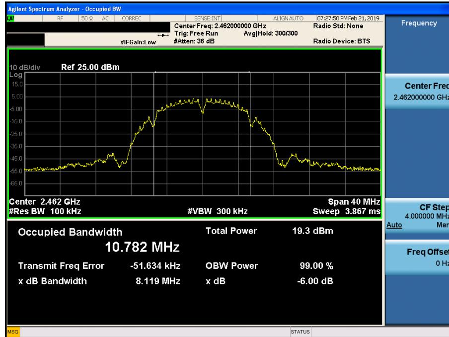
**6 dB Bandwidth****TM 2 & Lowest**
