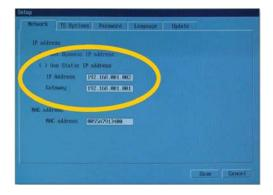
5 Click TS Option Tap -> Type the Host PC's IP address in the Terminal Server Network address from received the Router.
