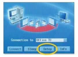
Click Network Tap -> Click Use Static IP Address-> Type in the IP Address and Gateway address of your a OfficeStation.
