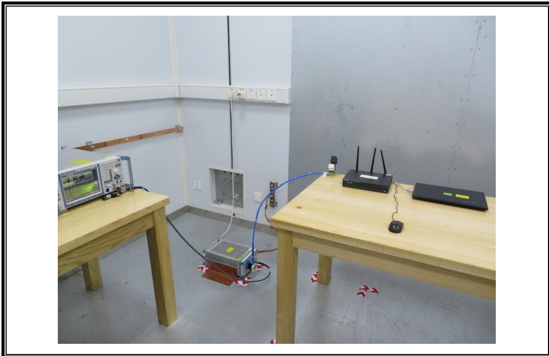
POWERLINE CONDUCTED EMISSIONS MEASUREMENT SETUP
