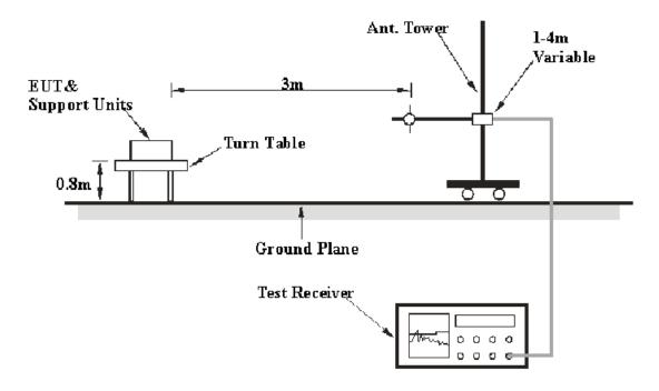
The radiated emission tests were performed in the 3 meters, using the setup accordance with the ANSI C63.4-2003. The specification used was the FCC 15.209 and FCC 15.247 limits.
