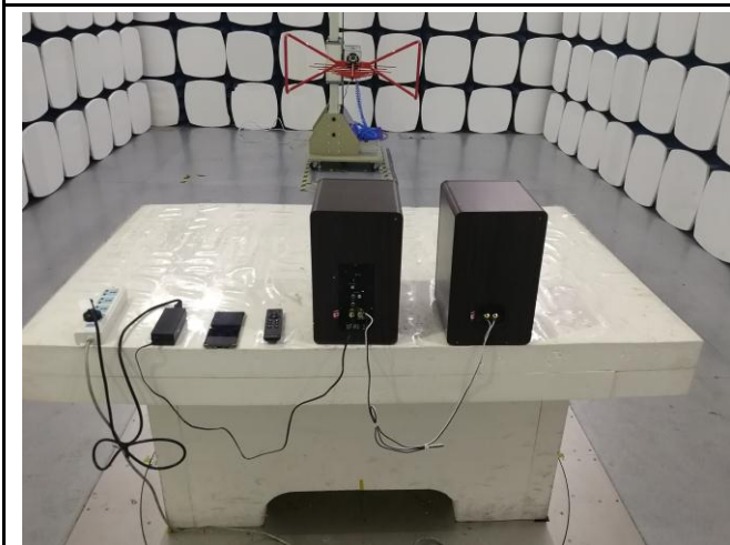
Conducted Emissions Test Setup Front View
