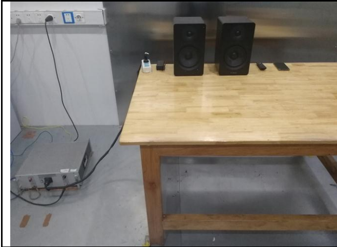
Conducted Emissions Test Setup Front View
