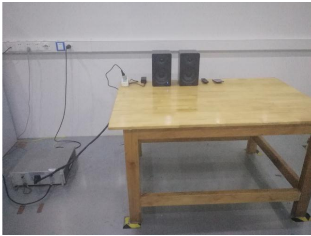
Conducted Emissions Test Setup Front View
