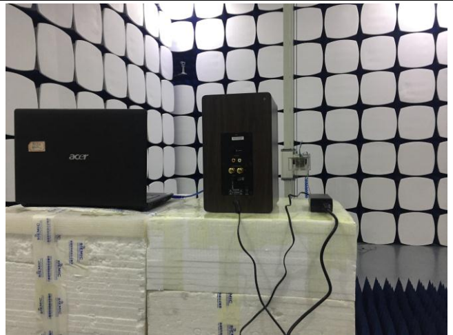
Radiated Spurious Emissions Test Setup Above 1GHz
