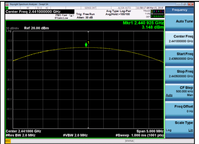
8DPSK Output power - Mid CH 2441
