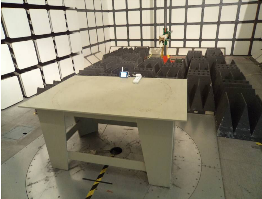
Radiated Emissions – Front View (1-25 GHz)
