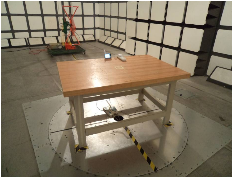
Radiated Emissions – Front View (30-1000 MHz)
