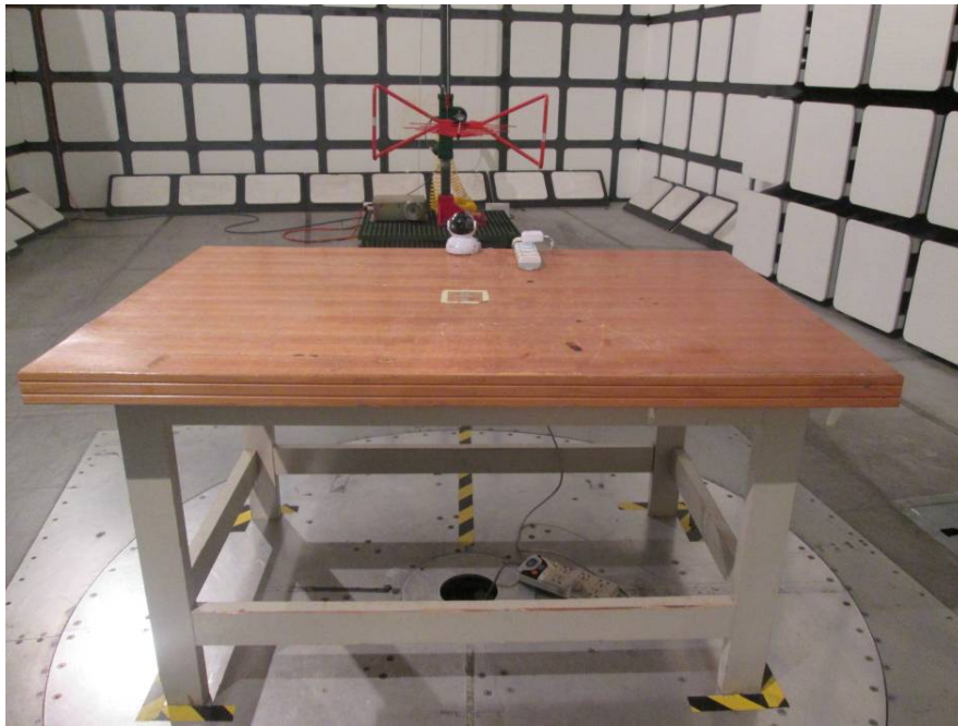
Radiated Emissions – Front View (30-1000 MHz)
