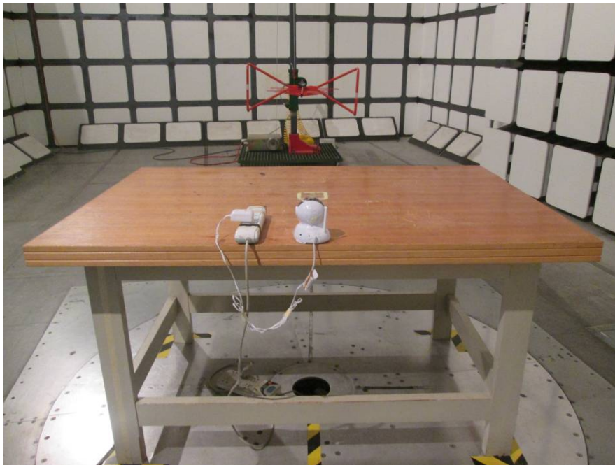
Radiated Emissions – Rear View (30-1000 MHz)
