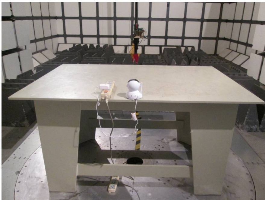
Radiated Emissions – Rear View (1-25 GHz)
