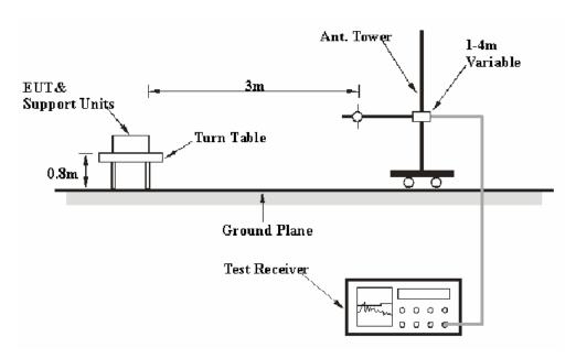
The radiated emission tests were performed in the 3 meters test site, using the setup accordance with the ANSI C63.4-2009. The specification used was the FCC 15.209 and FCC 15.247 limits.
