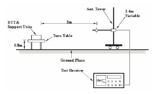
The radiated emission tests were performed in the 3 meters test site, using the setup accordance with the ANSI C63.4-2009. The specification used was the FCC 15.209 and FCC 15.247 limits.
