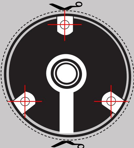
To wall mount the camera, drill three holes using 3/16" drill bit and the template.
