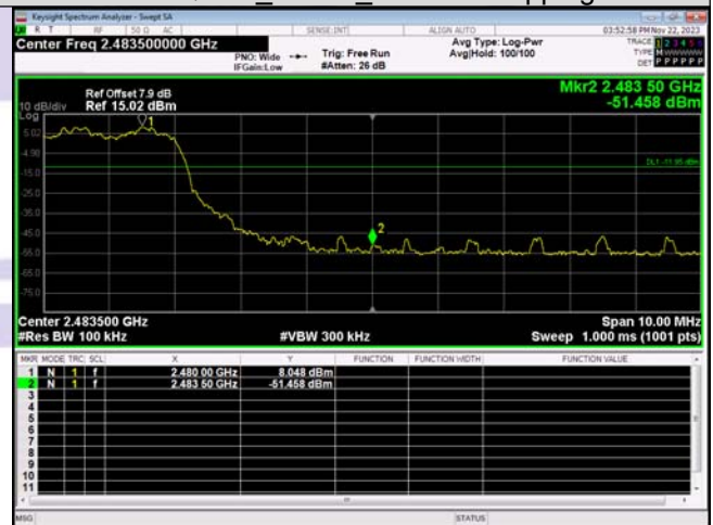
Out Of Band Emission(Left) \pi/4 DQPSK_2-DH1_Channel Hopping
