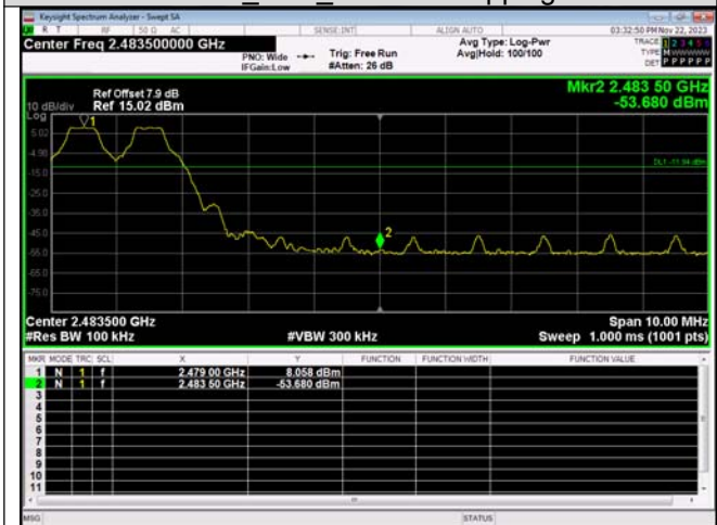
Out Of Band Emission(Left) GFSK_DH1_Channel Hopping
