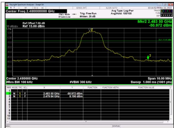
Out Of Band Emission 8DPSK_3-DH1_Channel 78
