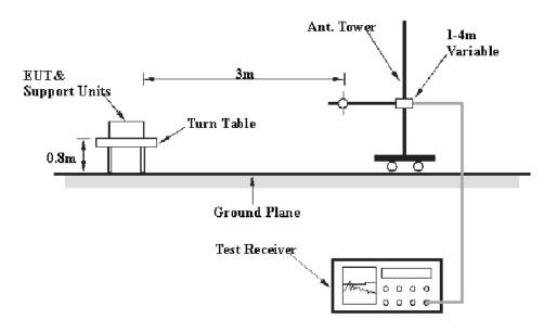
The radiated emission tests were performed in the 3 meters test site, using the setup accordance with the ANSI C63.10-2013. The specification used was the FCC 15.209 and FCC 15.247 limits.
