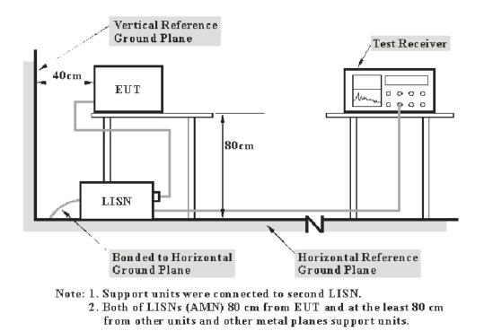
The setup of EUT is according with ANSI C63.10-2013 measurement procedure. The specification used was with the FCC Part 15.207 limits.
