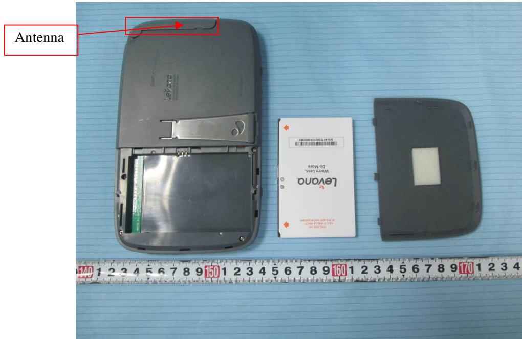
EUT – Cover off View 1
