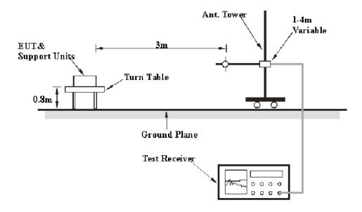
The radiated emission tests were performed in the 3 meters test site, using the setup accordance with the ANSI C63.4-2014. The specification used was the FCC 15.209 and FCC 15.247 limits.
