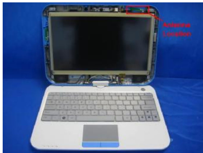
Picture 3 antenna positions
