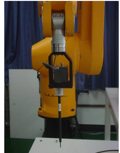
Picture6:ES3DV3 E-field probe
