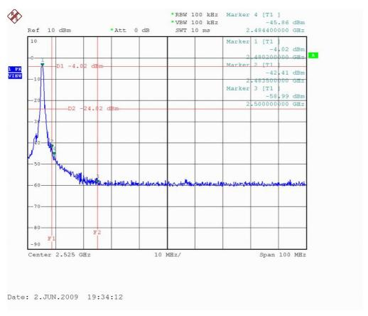
\*: The highest emission of f>2483.5MHz was detected at 2.4385GHz which below the 20dBc limit line.
