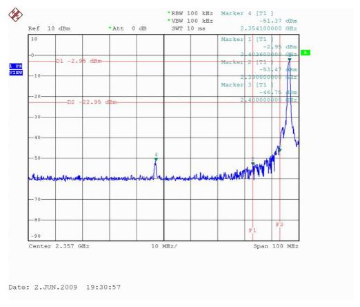
\*: The highest emission of f<2390MHz was detected at 2.3541GHz which below the 20dBc limit line.
