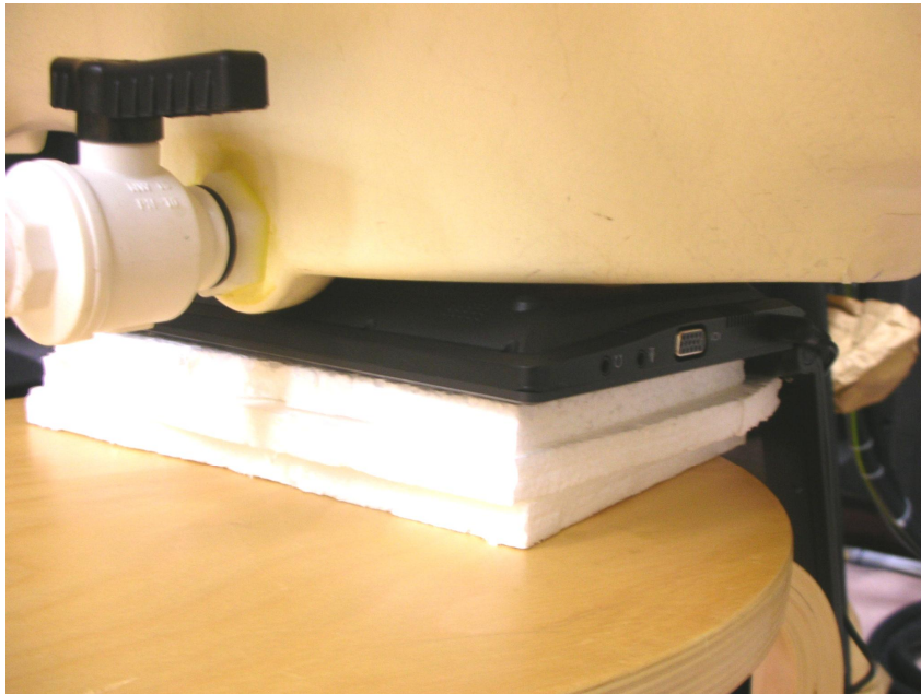
Below: SAR Test Close Position Setup At Flat Phantom
