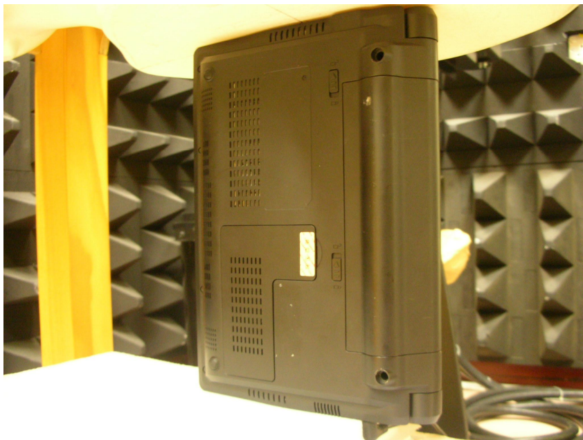
Below: SAR Test Close Position Setup At Flat Phantom
