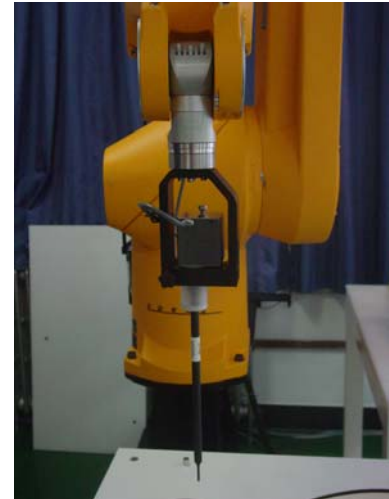
Picture6:ES3DV3 E-field probe
