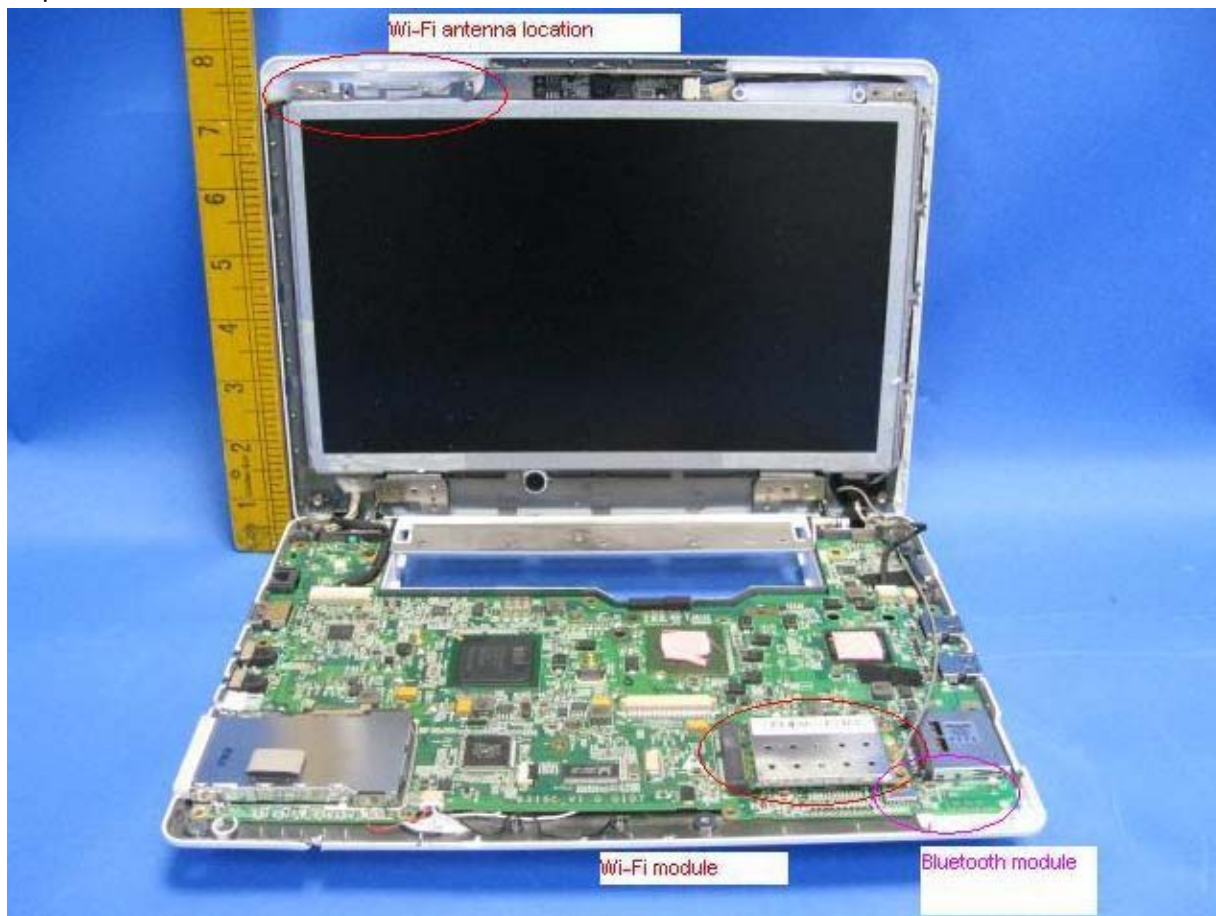
Picture 3 antenna positions
