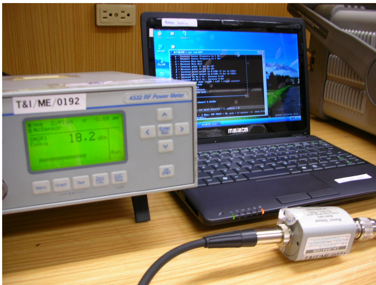
Conducted Power Measurement Test Setup - Closer View
