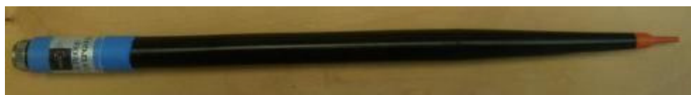
Figure 1 – MVG COMOSAR Dosimetric E-field Dipole
