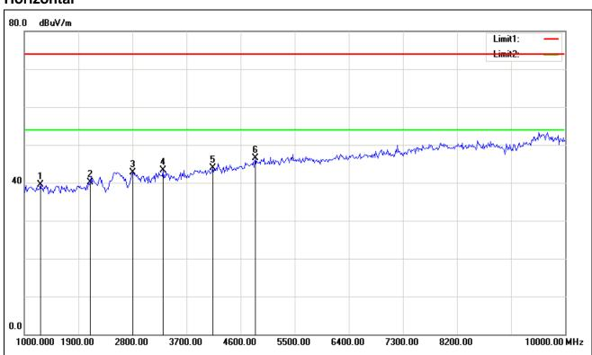
Test Mode: TX / IEEE 802.11n HT20 MHz (CH Mid) Tested by: Sam Zeng
