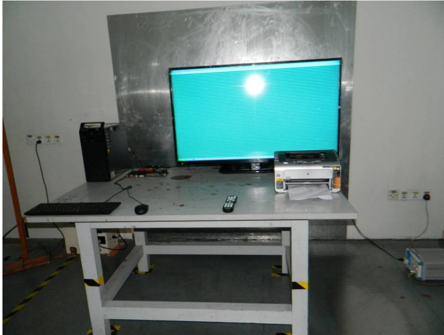
Photo of Power line Conducted Emission Measurement
