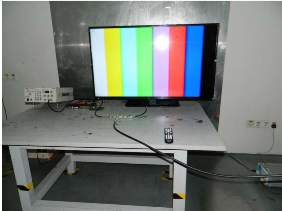
Photo of Antenna Conducted Emission Measurement
