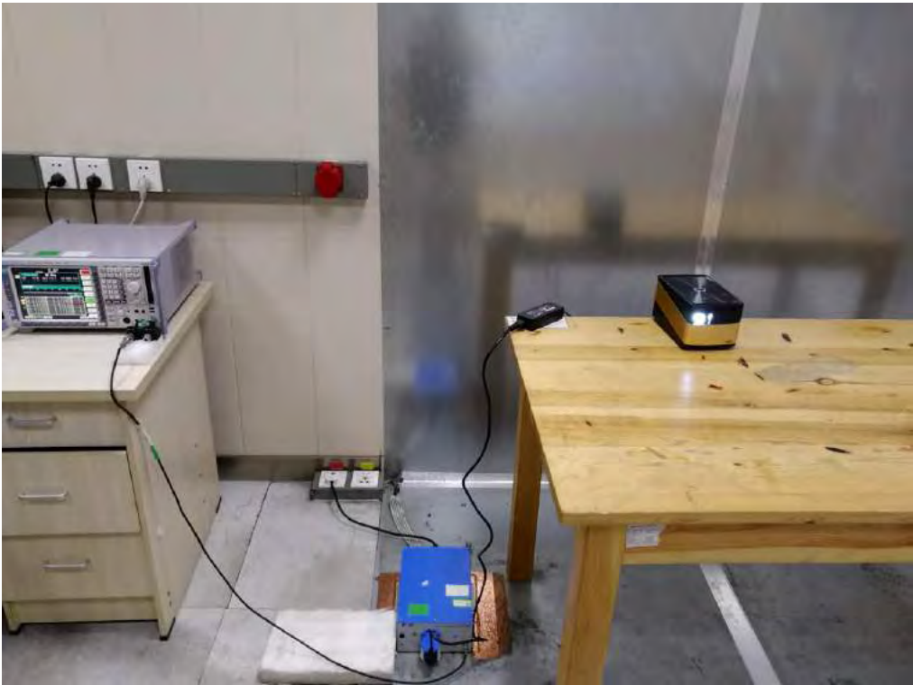
FCC RADIATED EMISSION TEST SETUP BELOW 1GHZ
