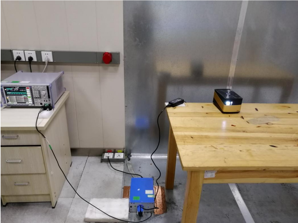
FCC RADIATED EMISSION TEST SETUP BELOW 1GHZ
