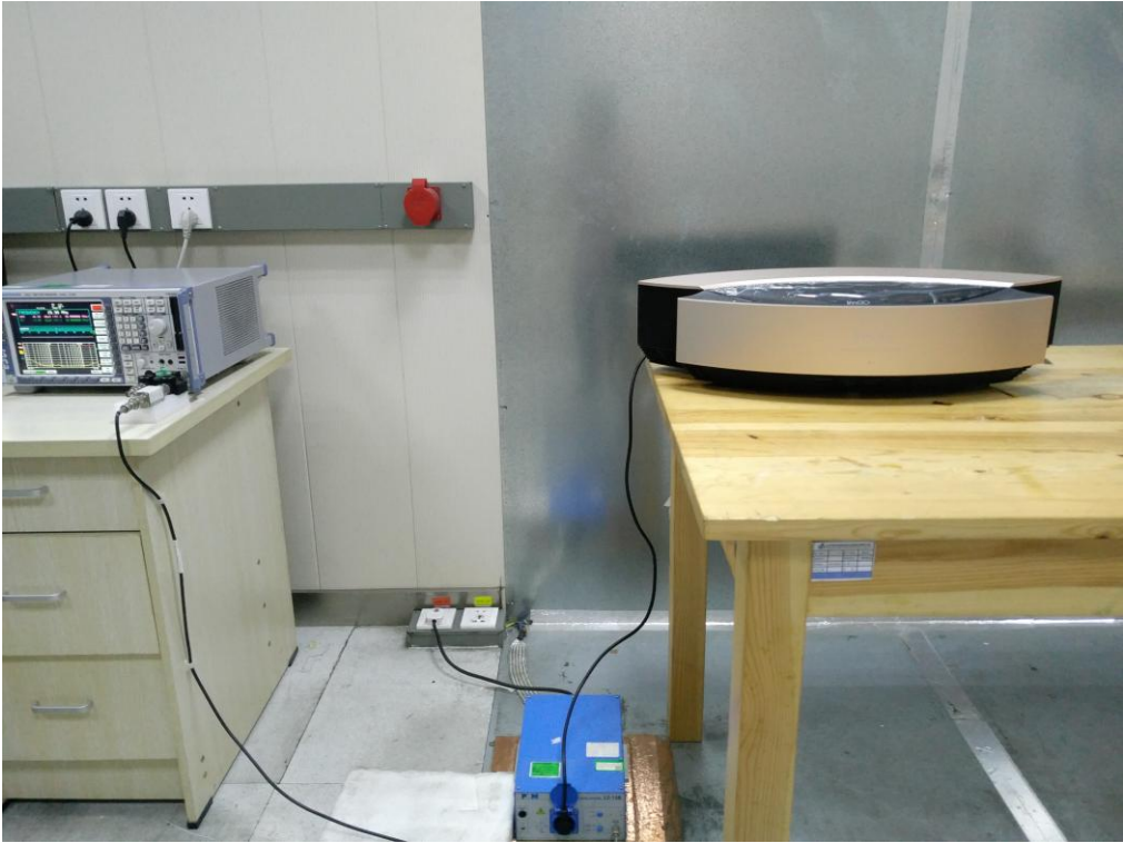
FCC RADIATED EMISSION TEST SETUP BELOW 1GHZ
