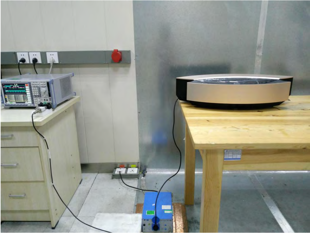
FCC RADIATED EMISSION TEST SETUP BELOW 1GHZ
