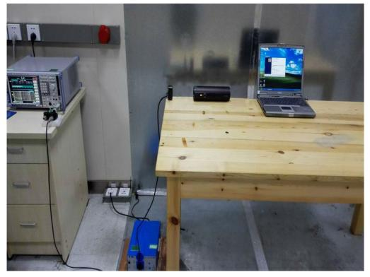
FCC RADIATED EMISSION TEST SETUP BELOW 1GHZ
