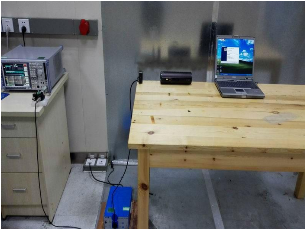
FCC RADIATED EMISSION TEST SETUP BELOW 1GHZ
