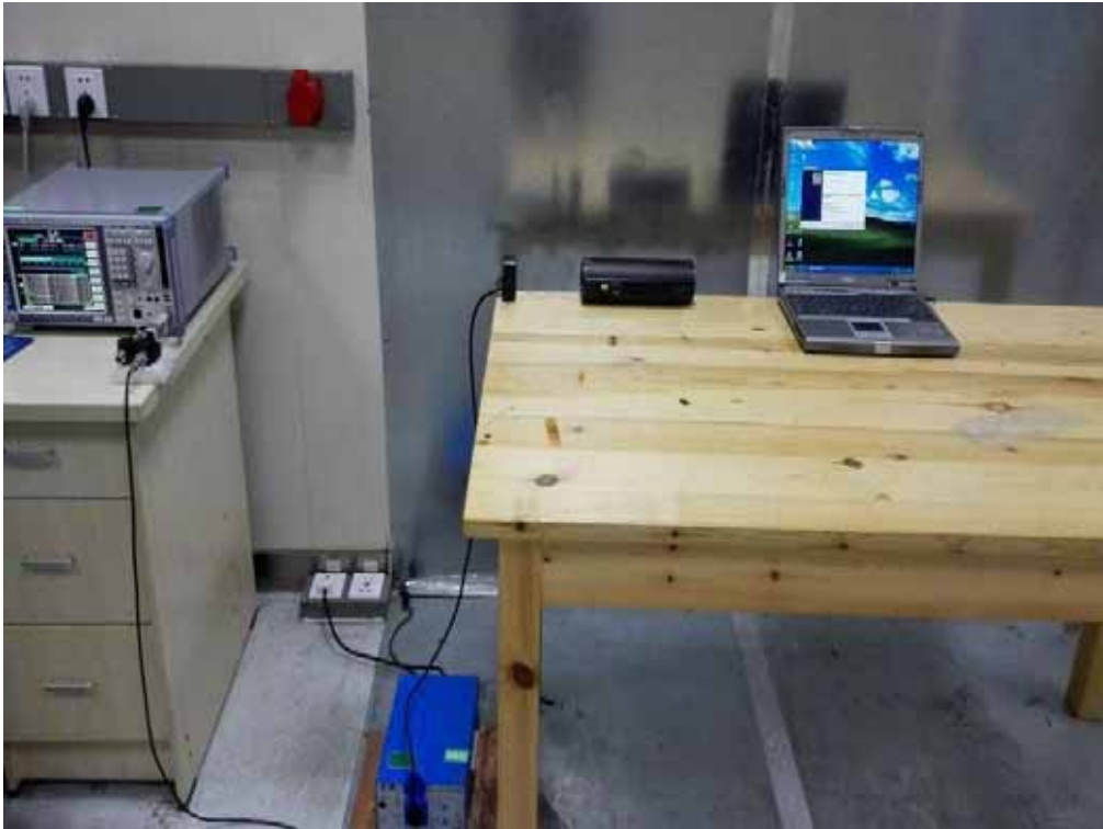
FCC RADIATED EMISSION TEST SETUP BELOW 1GHZ
