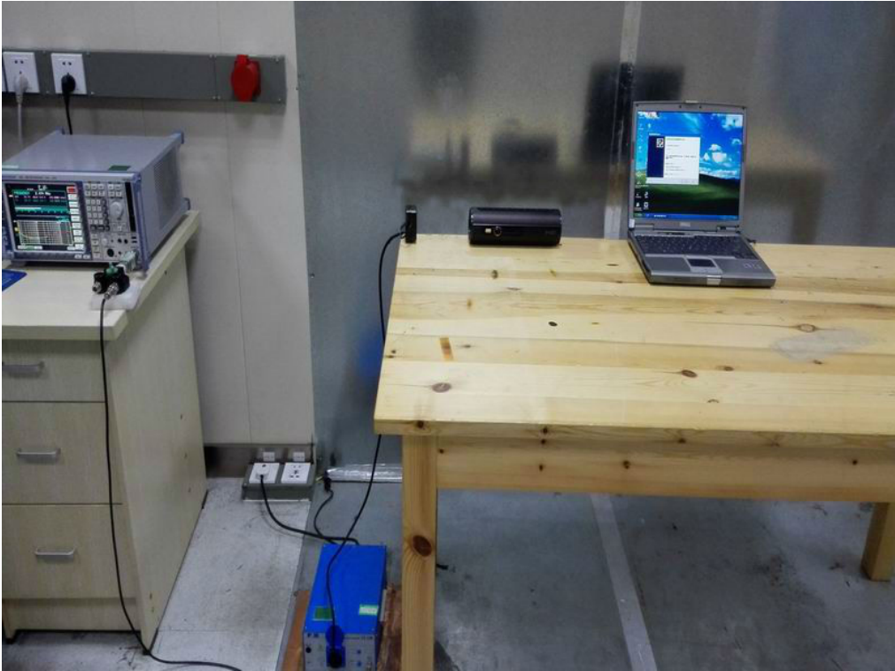
FCC RADIATED EMISSION TEST SETUP BELOW 1GHZ
