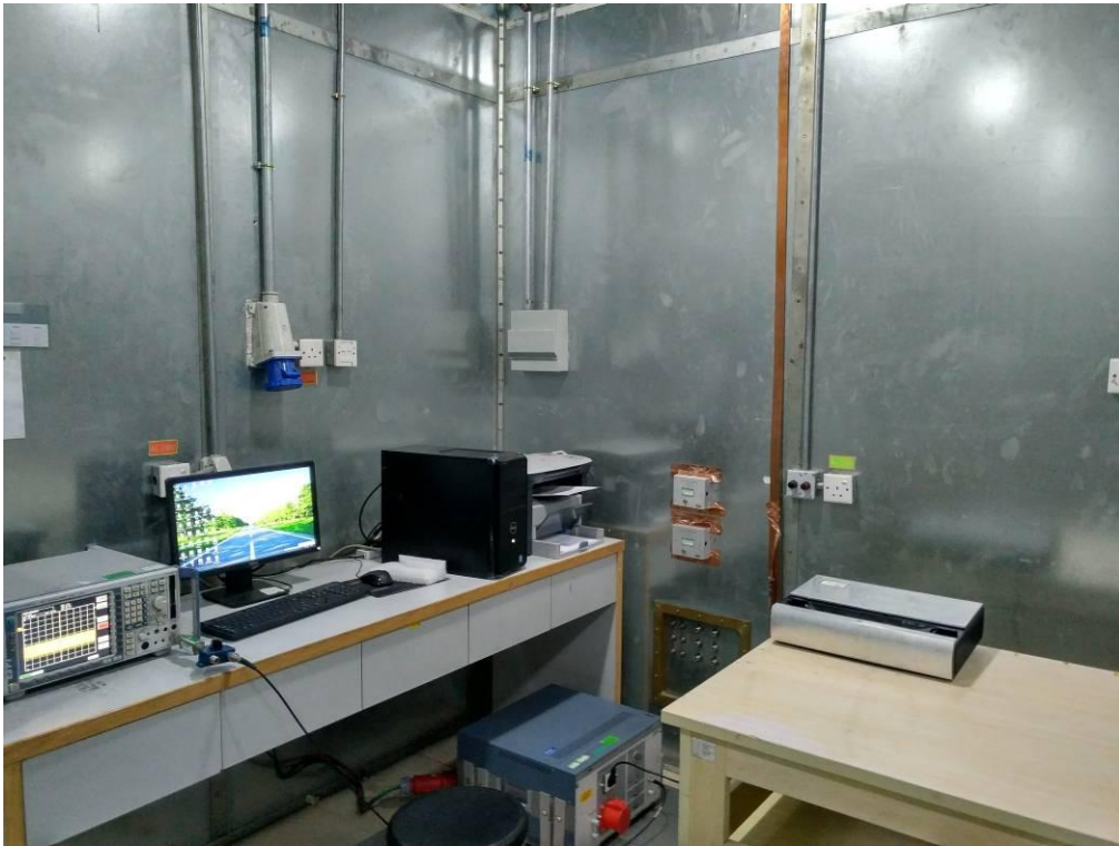
FCC RADIATED EMISSION TEST SETUP BELOW 1GHZ
