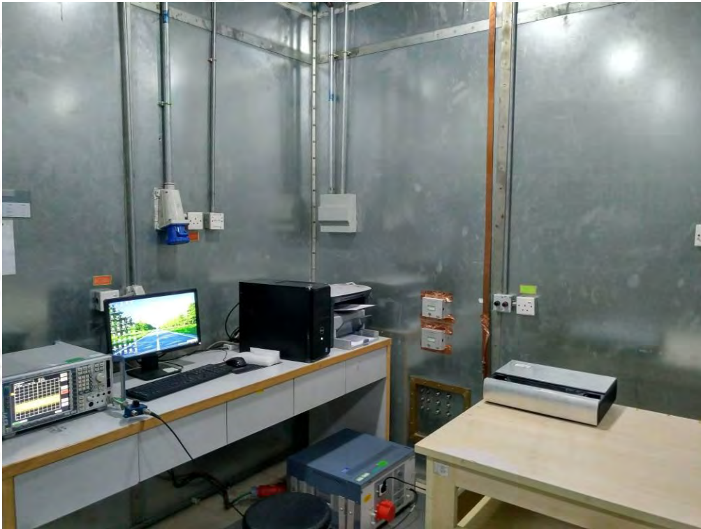
FCC RADIATED EMISSION TEST SETUP BELOW 1GHZ
