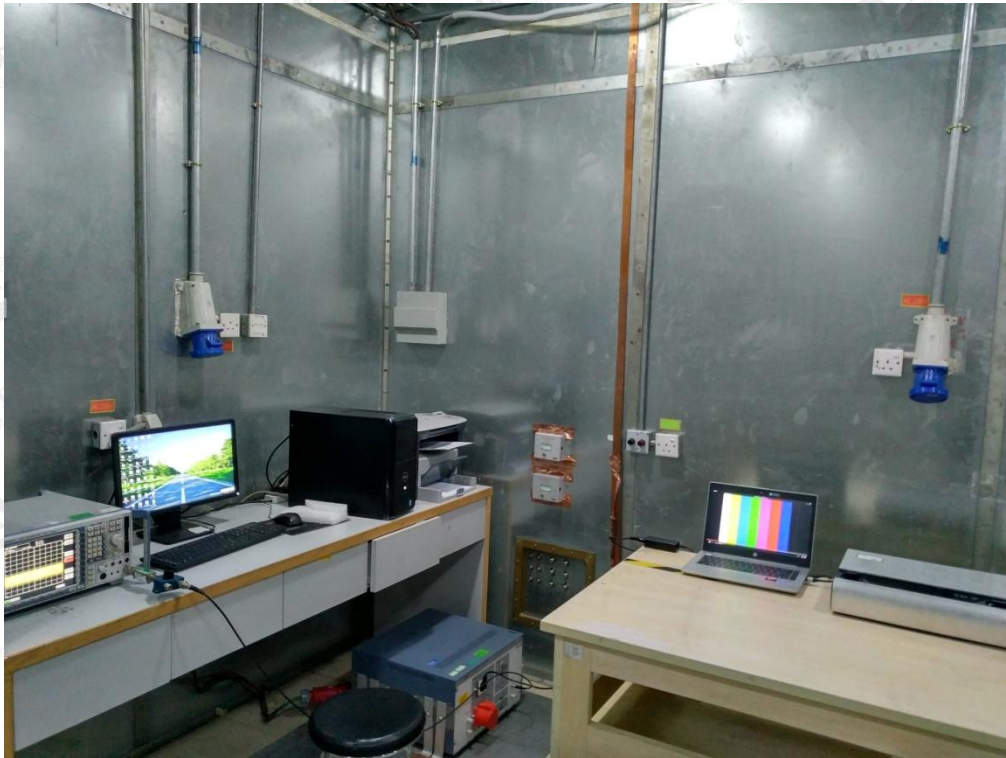
FCC RADIATED EMISSION TEST SETUP BELOW 1GHZ
