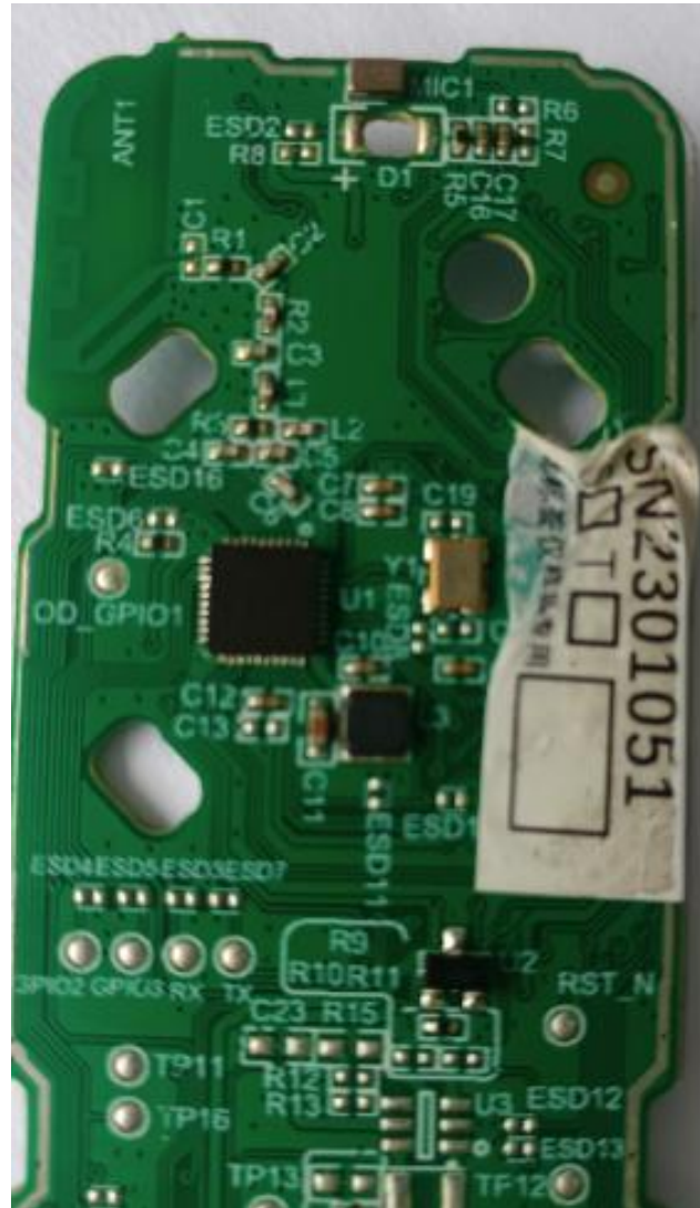
Antenna position diagram of new motherboard
