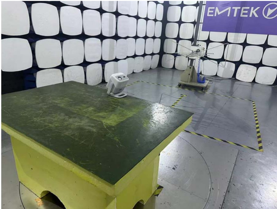
Spurious Emission Test Setup (Below 1GHz)
