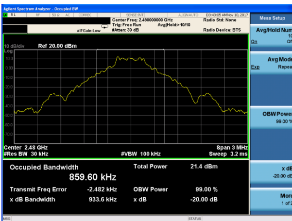
20dB Bandwidth plot on channel 78 (1Mbps)
