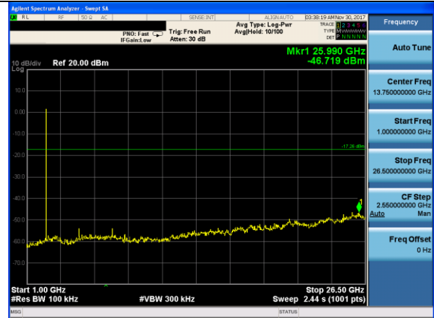
GFSK on channel 78
