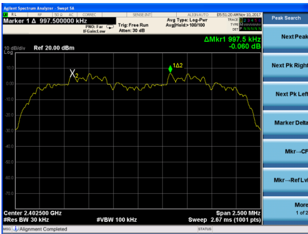
(3Mbps) Channel Separation plot on channel 39-40
