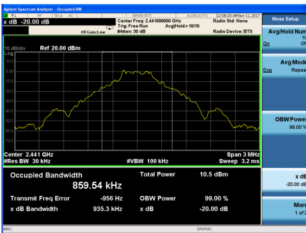
20dB Bandwidth plot on channel 39 (1Mbps)
