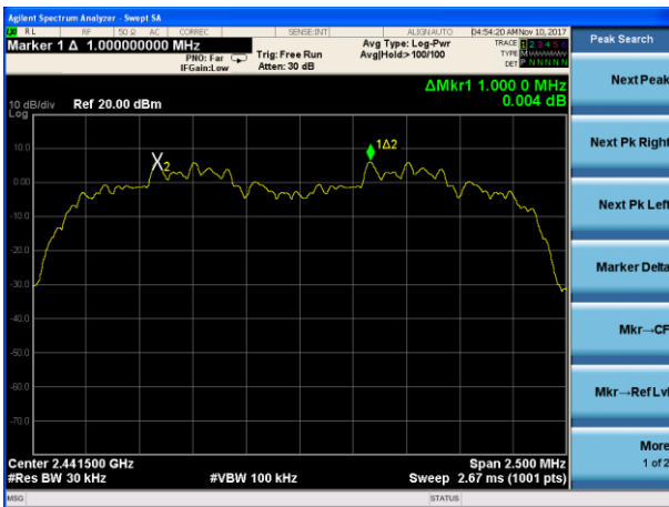
(3Mbps) Channel Separation plot on channel 77-78
