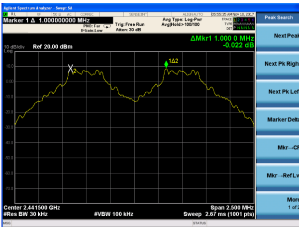
(1Mbps) Channel Separation plot on channel 39-40
