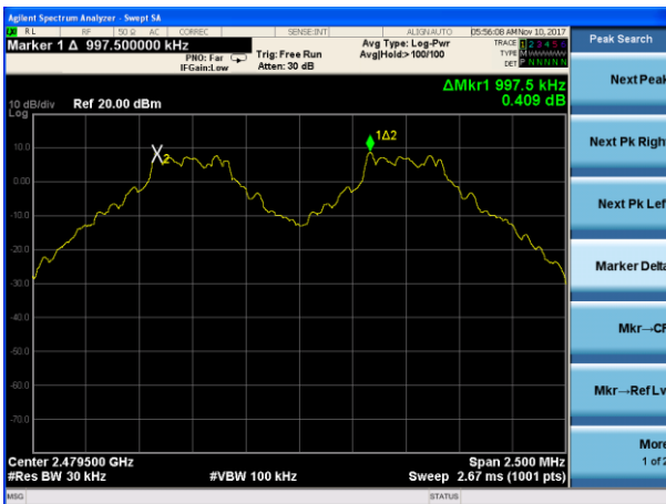
(1Mbps) Channel Separation plot on channel 77-78
