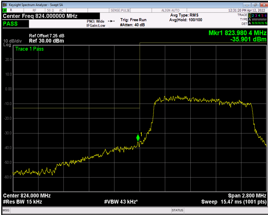
Band5 QPSK BW=1.4MHz Channel=20643 RB Size=1 Position=#Max NB Index=0
