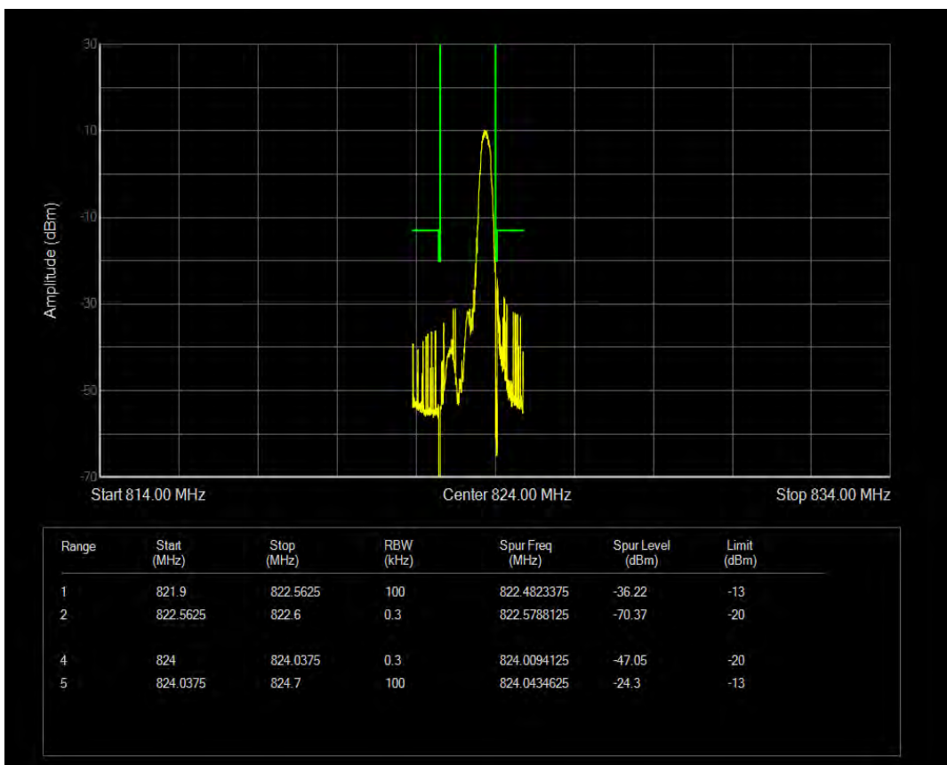
Band26(814-824) QPSK BW=1.4MHz Channel=26783 RB Size=6 Position=#Max NB Index=0
