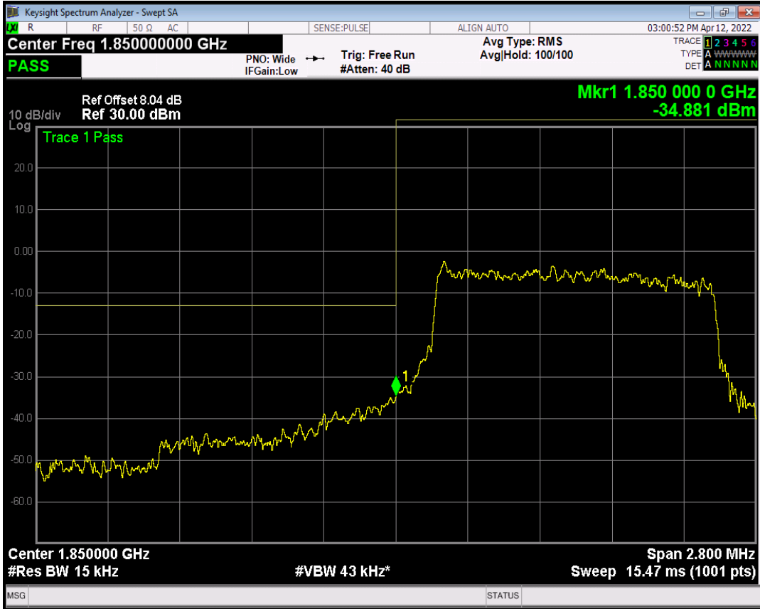
Band25 QPSK BW=1.4MHz Channel=26683 RB Size=1 Position=#Max NB Index=0
