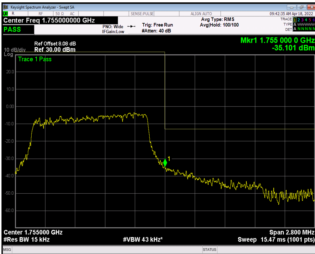
Band4 16QAM BW=10MHz Channel=20000 RB Size=1 Position=#0 NB Index=0
