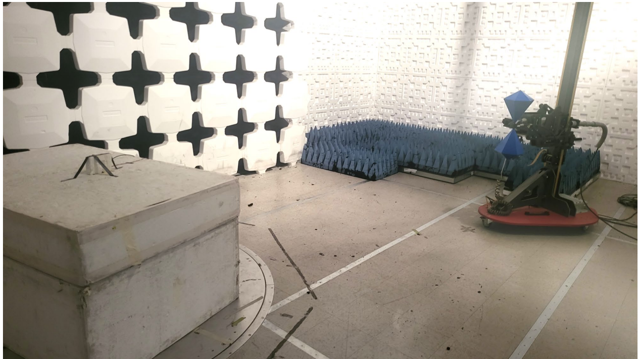
Figure 3. Radiated Emissions Test Setup (30 - 1000 MHz)
