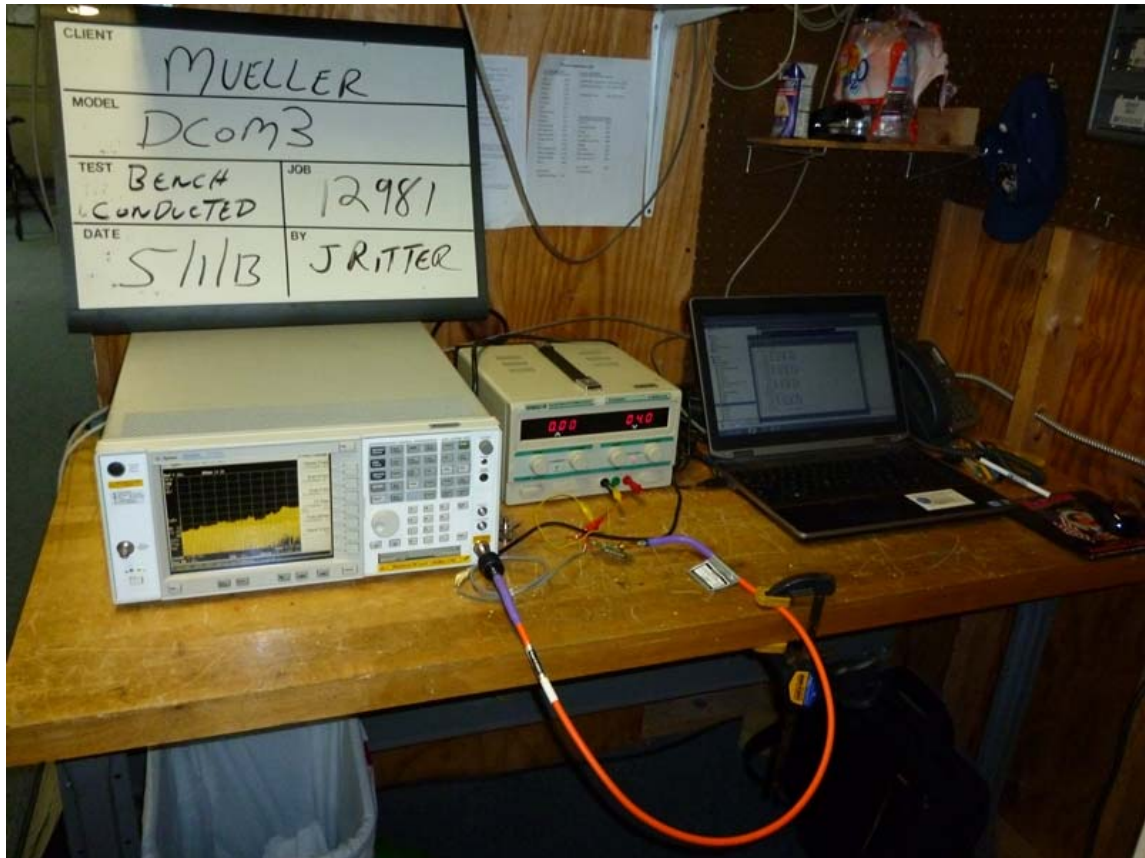
Figure 1-Conducted Emissions Test Set Up
