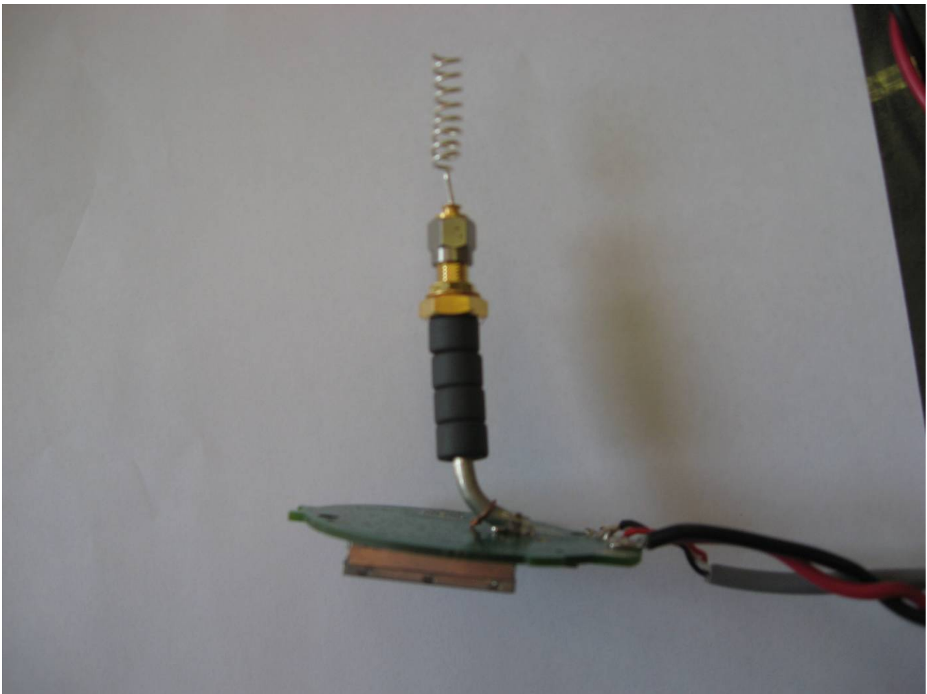
Photograph 1: DCOM3 with New Antenna
