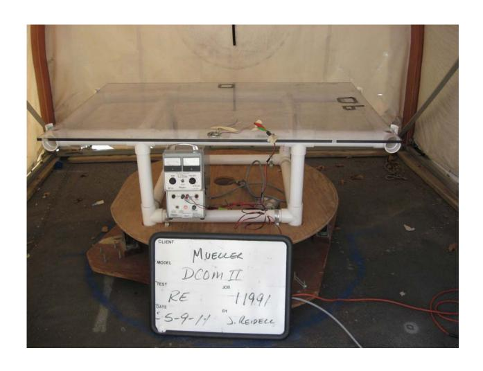
**Radiated Emissions Test Setup, Rear**
