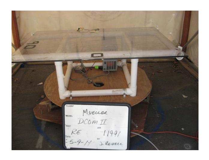
**Radiated Emissions Test Setup, Front**
