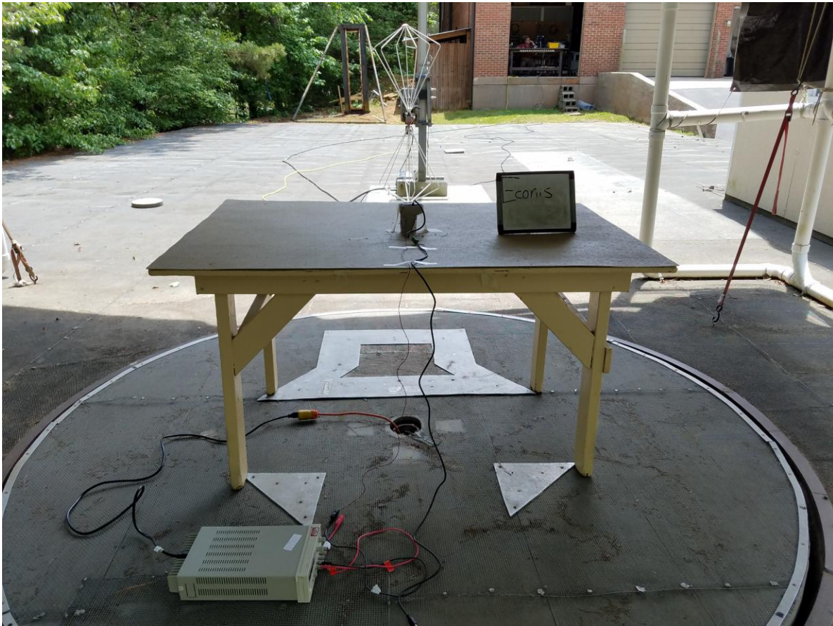
Figure 1. Radiated Emissions Test Setup – 30 – 200 Mhz
