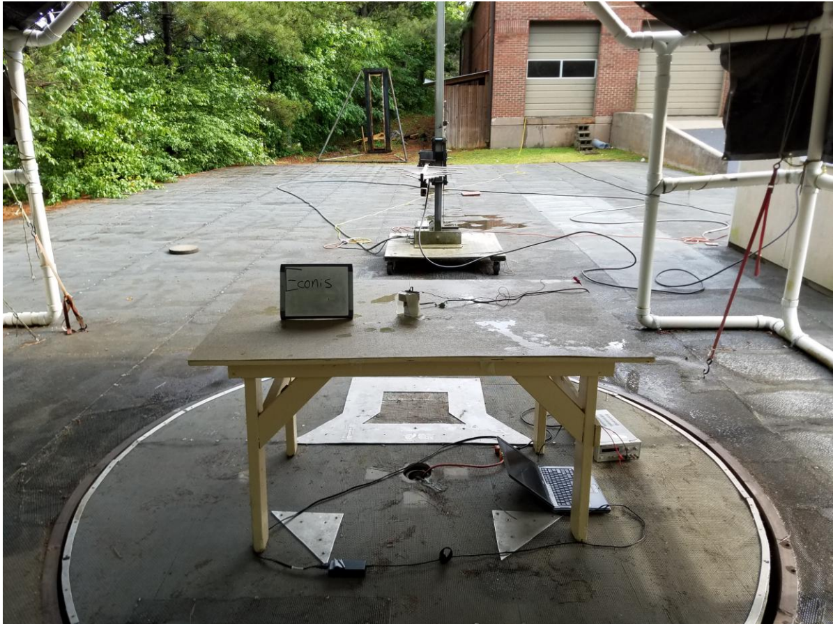
Figure 2. Radiated Emissions Test Setup – 200 Mhz – 1000 Mhz
